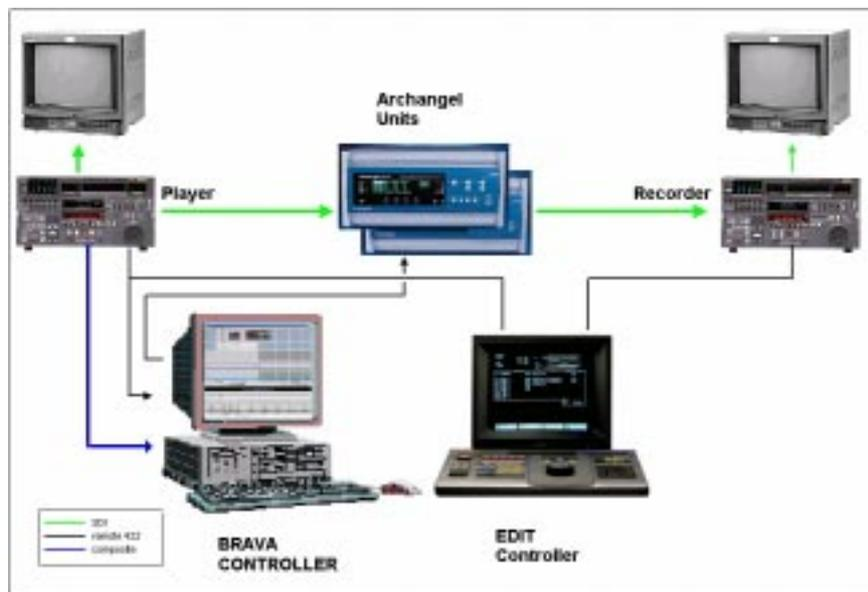
The Brava Real-Time Control in a tape-to-tape environment
