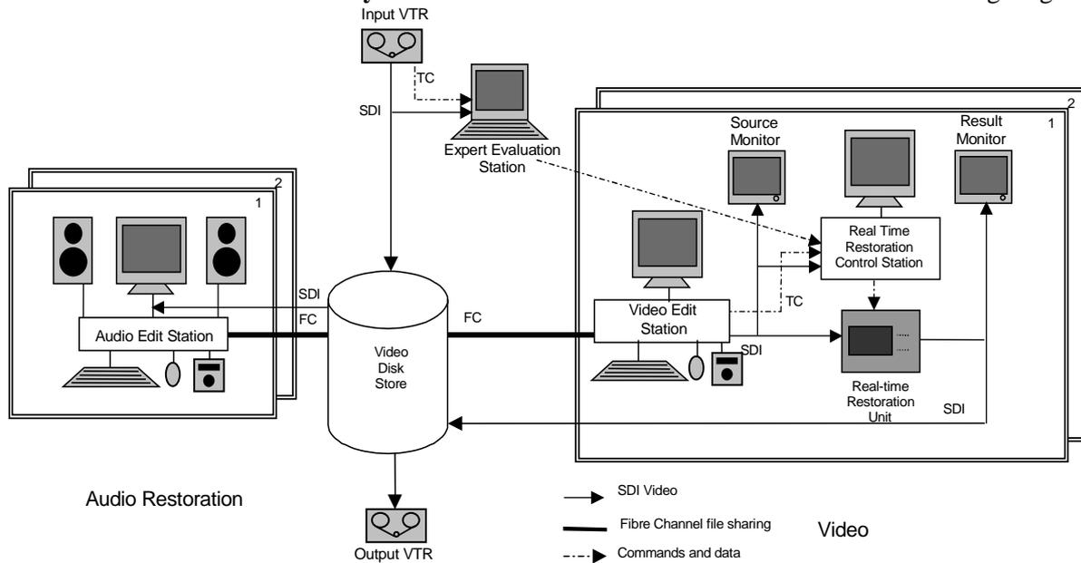
The principle is to replace the tape-to-tape editing system by a non-linear editing system, that additionally gives to the operator the following functionalities :
